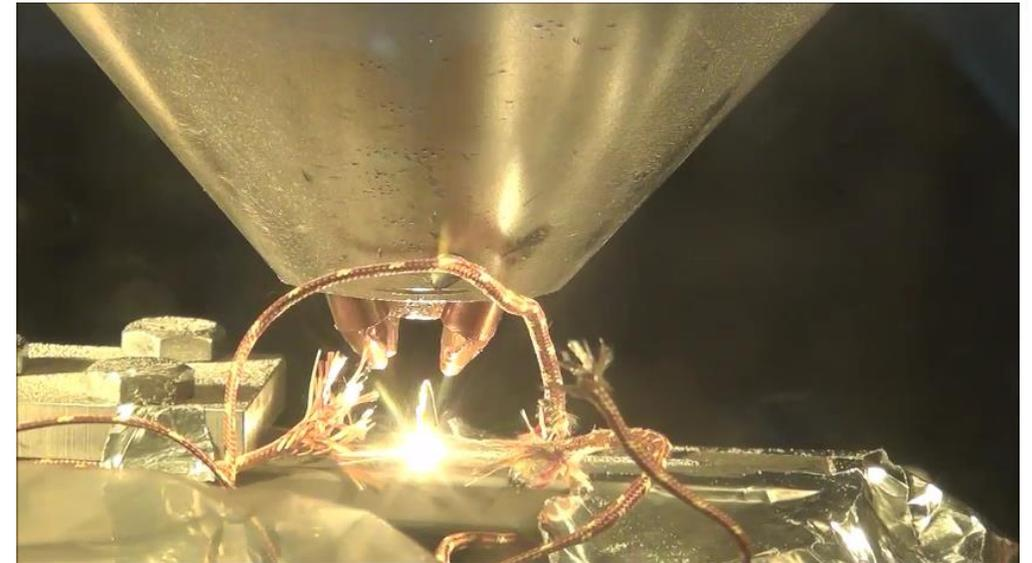
Both processes use a laser or electron beam, but the spot size in PBF is an order of magnitude smaller and moves much faster.
