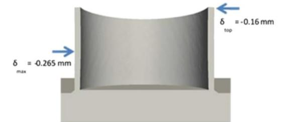
Fig. 13 Distortion of the tube with respect to nominal geometry after high speed machining
