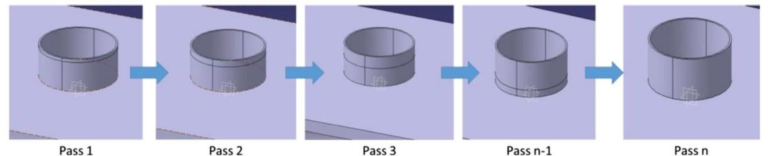
Fig. 9 Intermediate machined geometries
