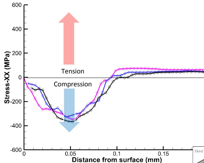
For this material, the cutting process generates a significant amount of stress near the surface.
