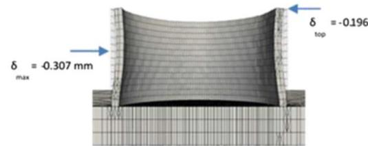
Fig. 11 Distortion of the tube after laser cladding with respect to the nominal geometry
