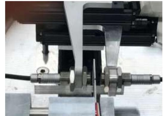
Eddy current sensors for displacement measurement
