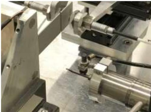
High speed fluted cutting tool for producing slit in fuel plate
