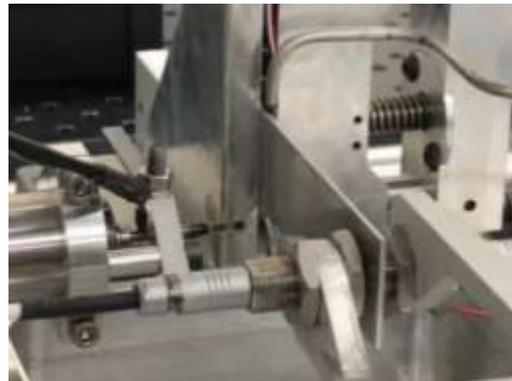
Video showing surrogate fuel plate slitting on wet system during comparison test
